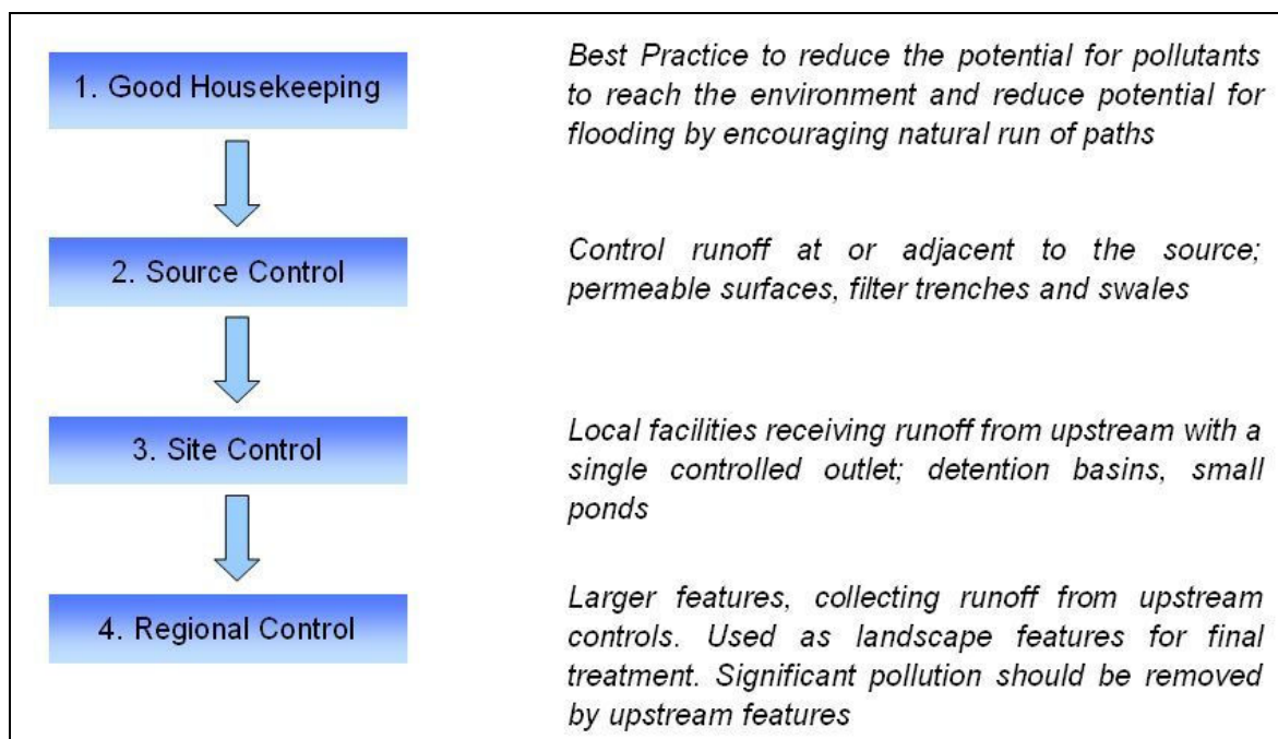
Figure 5 – SuDS treatment train (source: Peterborough Surface Water Management Plan Strategic and Intermediate Assessment Report).
